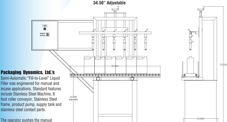
The operator pushes the manual container stop out, moves the containers to be filled along the roller conveyor surface into position under the nozzle bar assembly and pushes the cycle start button. Upon completion of the fill cycle the nozzle bar assembly automatically returns to the starting position. It's as simple as that.
