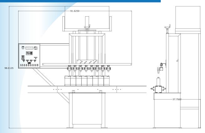
The **Packaging Dynamics**, **Ltd**. Automatic Time-Gravity Straight-Line Filling System Model SLA-TG is constructed of stainless steel that provides for easy clean ups and maximum chemical resistance. Engineered to time-fill liquids into containers as small as 2 oz. or as large as 2.5 gallon containers. Rates range from 12 to 60 containers per minute depending on the container size and product viscosity.
