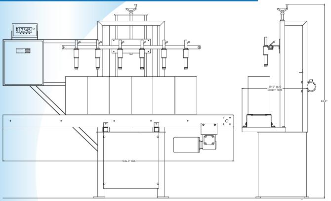
Packaging Dynamics Ltd. introduces the Mass Flow Liquid Filler which utilizes Micro Motion Coriolis flow meter mass technology. The Coriolis flow meters measure mass directly and therefore are insensitive to changes in process conditions or fluid composition. The systems meets performance requirements of manufacturers in the cosmetics, pharmaceutical, food and beverage industries. These requirements include accuracy of +/- 0.5%. Product viscosities vary from water to 40,000 cP with
